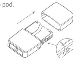
2. 0.9 mL liquid maximum fill. Press the silicon stopper back into the hole for a proper seal.
